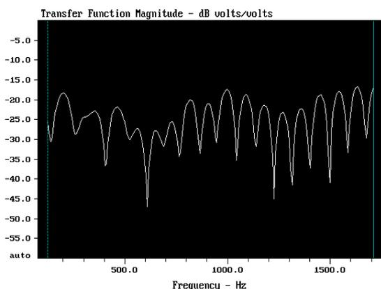
**Region d:** "Late-Early-Reflections". No reports of Box-Klangfarbe was given due to introducing reflecting surfaces with a time-delay in this region. The TOR-FFT-analysis including this time region shows only additional small "ripples" to the main "envelope" created by the reflections in the earlier parts. When we increase the time delay of the reflection further, we enter the "time-domain"-region of sound-perception, and a "lonesome" reflection will be perceived as echo, not as coloration.
