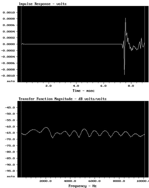
The Comb-Between-Teeth-Bandwidth from this "mixing console-reflection" is some 800 Hz. Examples of other comb-filters are given in the Appendix. (Multiple Reflections etc.)
