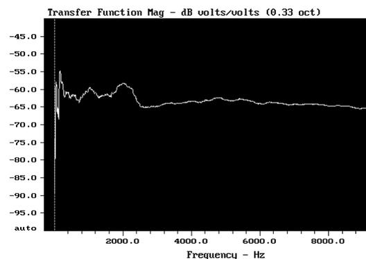
Psycho -acoustic studies (see part 4 +5) indicate that coloration is formed in the first part of the sound. For this sound control-room, it is therefore interesting to investigate the FFT of the direct sound + the first reflection (localised to arrive from the mixing console). Therefore, we will "zoom in" on the part of the Imp. Resp. before the cursor in the figure above, and perform a FFT for this time window:
