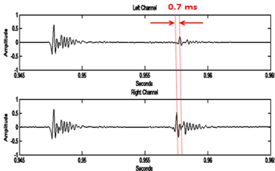
Fig. 2. Waveform of a recorded click with binaural simulation of a reflection from the right side of the (simulated) head.
