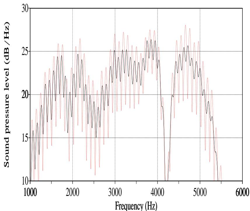
Fig. 3. Frequency analysis of a recorded click with binaural simulation of a reflection from the right side. Black= Left ear. Red/dotted=Right ear.
