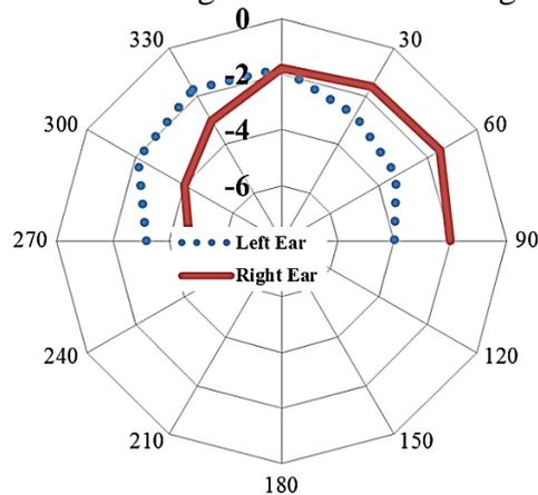
Fig. 6 Directivity of the ear(s) measured from the Pd/binural patch
