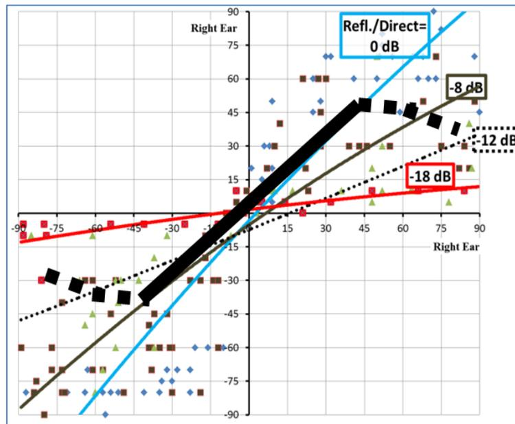
Fig. 5. Suggested curve for detectability of reflectors from surfaces at different angles ( $0^{\circ}$ =surfaces in front of head)
