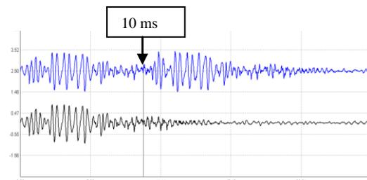
In the blue, upper curve, we see the 10ms delayed reflection that gives a combfilter with “comb-between-teeth- bandwidth” of  $1/10\text{ms}=100\text{ Hz}$ . A zoom-in shows this even more clearly:
