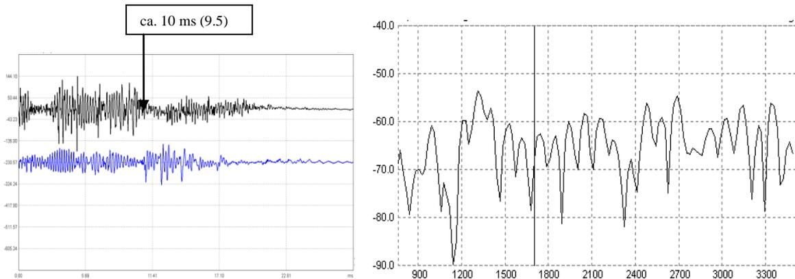
The clicking was not performed in exactly the same way in these two recordings (and the levels are not normalized). Looking at the frequency response above, we see a comb for the situation with the reflecting plate. The following zoom-in shows the frequency response With reflecting plate in Black, giving the comb, and Without reflector, showing no comb.
