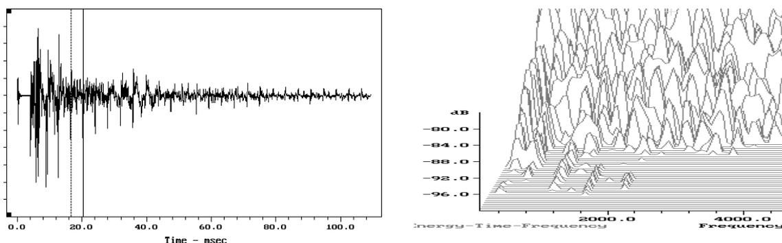
The frequency-response/-waterfall-curves show resonances giving the almost “ringing” sound observed when walking through the “naked” corridor. In [5] it is shown that even modest “scattering” treatment placing paintings/”posters” on the sidewalls reduced this combfilter/resonances and the “box-klangfarbe”.
