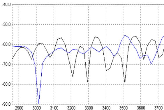
*(When we look more in detail into the curves, we see that the Comb-Between-Teeth (or peak-to peak) is somewhat higher than the intended 100Hz. This actually shows that the exact delay was not 10ms, but some 9.5ms, and the position was measured again afterwards, giving some 1,65m instead of 1,7m.)*
