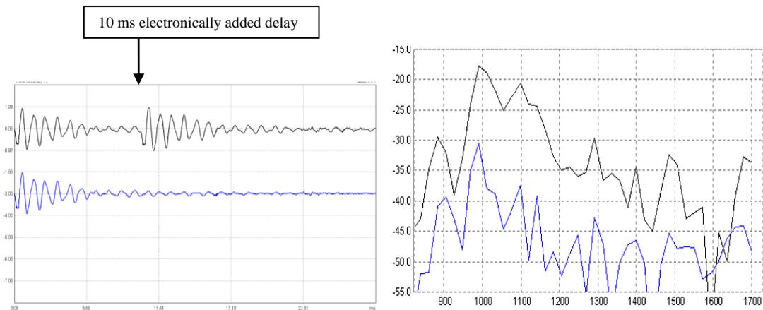
We see that the “centre frequency” of the Tongue-Drop is somewhat lower than for the Click Type A and B. There are signs of Combs for the Tongue-Drop, but perhaps not as clear as for Clicks Type A, B and C.
