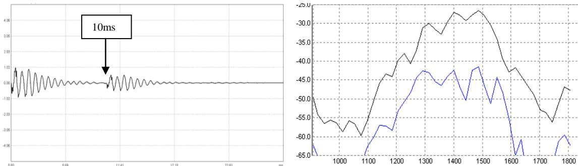
Here we see some comb-like structure for the upper curve (with delay), but not as clear as for type A and B. Also listening to Type C clicks with/without delay/reflector does not give as clear change in timbre as A and B, but the (very small) additional length is actually perceived!
