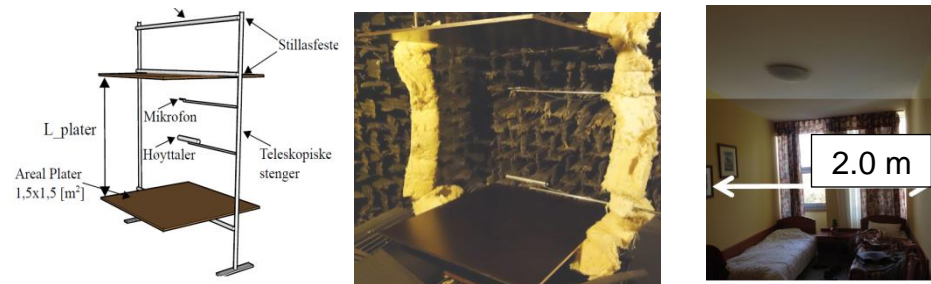
Figure App.A.2: Set up for measurements of flutter in anechoic chamber and hotel room
