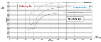
The figure above shows the build-up of a "continuous", long sound prolongs the attack, most clearly for the absorbent and transparent box (without close reflections). Close reflections (Reflecting box) shorten the "rise time" and gives less "smoothing" of the attack.
