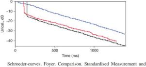
Schroeder-curves. Foyer. Comparison. Standardised Measurement and two In-Ear-Mic. Upper (blue): Standardised measurement Middle (red): Handclap, Lower (black): Tongue-drop.
