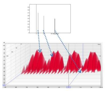
This situation also goes for the early reflections in a concert hall: The first reflections will give a coloration that influences the later ones. Also: the later comb filters will be narrower and narrower, with CBTB's much smaller than Critical Bandwidth, so that they do not give perceived coloration in the same way as the earlier reflections, as a gradual evolution towards diffuse field.
