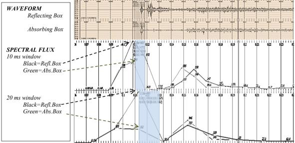
From these analyses, we clearly see that the (changes in) spectral flux is larger for the black curves/Refl.Box. Some other alternative methods for analysing spectral flux show results that are somewhat more unclear.
