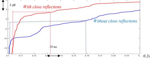
We see that the overall attack is faster with the close reflections. If we should want to measure the Steepness, we would need to closely define which part of the curve is interesting (especially for the blue curve). Quick estimations of Rise Time (to -5dB) gives:  $TR_{WithCloseReflections} = 30ms$ , and
