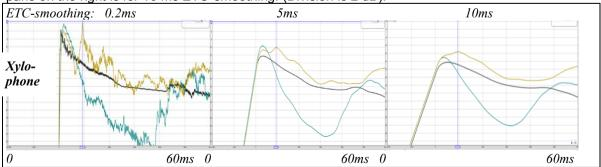
This figure clearly shows the importance of the decisions we have to make when analysing small differences in short attacks. If we assume that our ear has an integration time of 10 ms (or more), the setting with close reflections, *Refl.Box*, will be perceived with the "clearest" attack.
