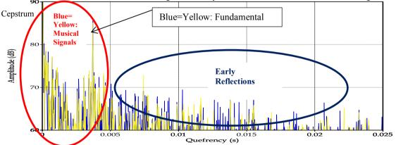
The high peak common for both blue and yellow corresponds to the fundamental  $(1/f_o)$  of the tone repeated most frequently. For lower quefrencies (in the red circle), the measured cepstrum values represents overtones and other "musical" frequencies in the signal and in this region, the results are the same for blue and yellow. For quefrencies between some 5 and 20 ms, the blue curve shows that there are early reflections. This was a very simple test, (and we knew the answer), but this shows
