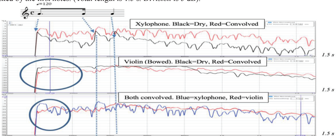
Figure 7 – Analysis of xylophone and violin playing the same music. Dry and convolved with long RT
