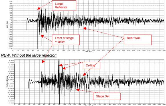
We see that the new, small reflector does not give a clear reflection from the pit to the stalls, but opens up for the later reflections from the ceiling etc.
