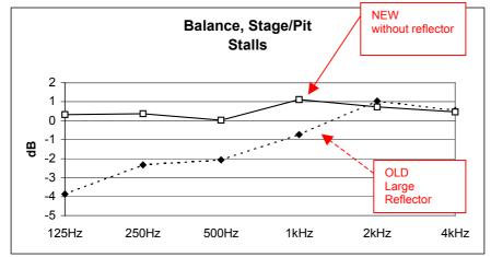
This figure shows that the stage/pit balance is improved, but still somewhat lower than what one would want for opera houses. The change is increasing with decreasing frequency. This might be due to that the large/old painted canvas reflector probably acted as an absorber for lower frequencies. More results on the G-parameter are given in App. 3.
