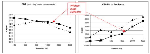
(EDT-results below 500 Hz might be somewhat insecure due to the measurement chain for the first measurements).
