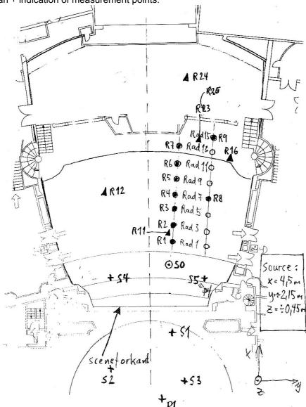
is seated at one large balcony with 12 rows, and the stalls have 17 rows, 4 of which are under the balcony. The volume is about 6500 m<sup>3</sup> thus giving 6.2 m<sup>3</sup>/seat. Plan + indication of measurement points:
