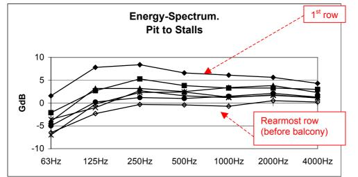
The following figure shows energy spectra in the stalls for a pit-source (after the removal of the large reflector), taken from seven positions positioned as an array parallel to the room's length-axis.
