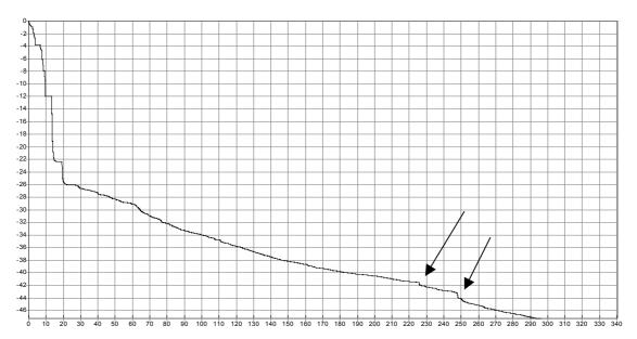
The reflections giving the echo are a combination of the reflection from the slightly curved rear wall directly (225msec) and from the rear corners (250msec). Some reflections from the "chandelier+ceiling", arriving a bit earlier "disturbs" the Impulse Response somewhat, but the echo is still clearly perceived, both in the house and in the listening tests of the impulse response.
