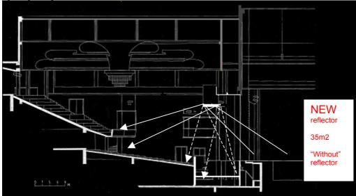
This section shows the "NEW", much smaller, flat, slightly diffusing wooden reflector underneath a lighting bridge:
