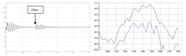
Here we see some comb-like structure for the upper curve (with delay), but not as clear as for type A and B. Also listening to Type C clicks with/without delay/reflector does not give as clear change in timbre as A and B, but the (very small) additional length is actually perceived!
