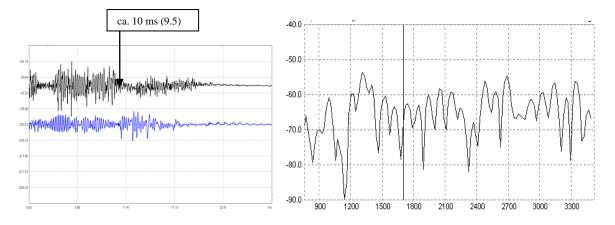
The clicking was not performed in exactly the same way in these two recordings (and the levels are not normalized). Looking at the frequency response above, we see a comb for the situation with the reflecting plate. The following zoom-in shows the frequency response With reflecting plate in Black, giving the comb, and Without reflector, showing no comb.
